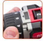
If your drill has a drill and clutch mode, set it to clutch mode. Set your drill to 30% of maximum torque.
