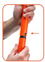
Turn the upper tool body clockwise to lock it into place.
