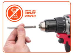
Insert the T-15 driver bit into your drill. Do not use an impact driver.
