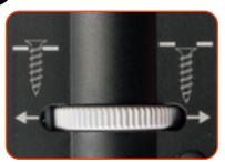
Before fastening on the deck top, drive a few screws into a scrap piece of material and adjust the depth set dial accordingly. For Edge screws, sink them 0-6mm below the surface of the deck board.
