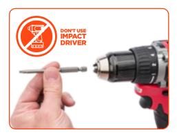
Insert the T-15 driver bit into your drill. Do not use an impact driver.
