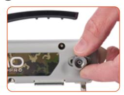
Adjust the spacer teeth on the tool with the thumb dial to fit your board.
