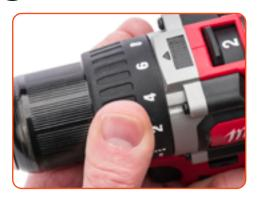
If your drill has a drill and clutch mode, set it to clutch mode. Set your drill to 30% of maximum
