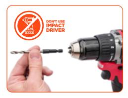
Speed up the job by attaching the pre-drill bit to another drill.\*
