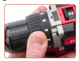
If your drill has a drill and clutch mode, set it to clutch mode. Set your drill to 30% of maximum torque.
