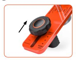
Adjust the stop block to the proper joist width and tighten the knob.
